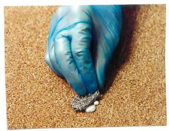
6) You will see the mercury filling the gaps between the metal strands as it forms an amalgam.
