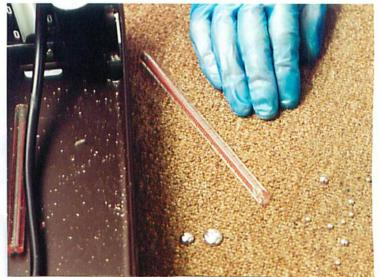
2) Using the scoop, push the globules of mercury together so that they form large globules which can be collected using the syringe.
