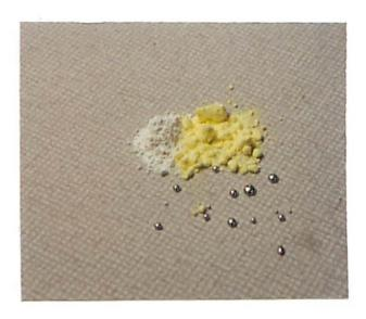
6) Using the scoop, mix the powders with the spilt mercury
