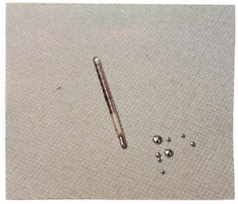
2) Using the scoop, collect the mercury globules together so that they merge into larger globules.
