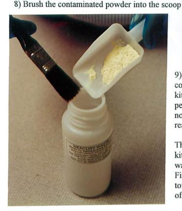
9) and place it in the waste container. Cap the waste container tightly and replace the items in the spillage kit case, until it is needed again. Unless the same person will be using the spillage kit each time, do not replace the mask and gloves, for hygiene reasons.
